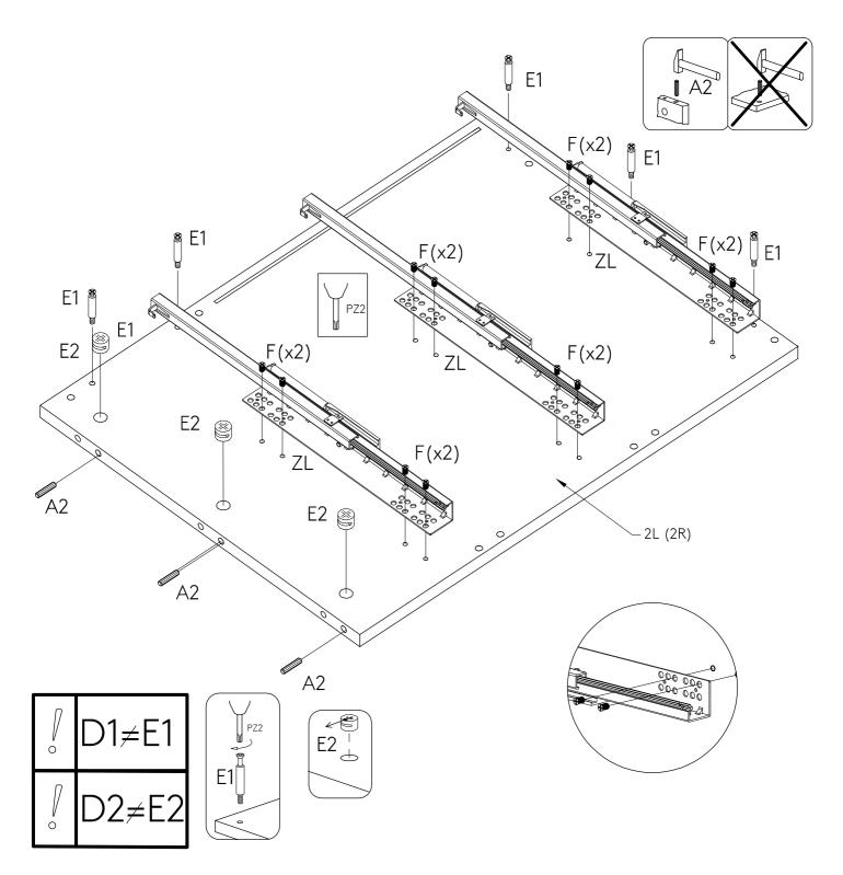
**STEP 5:** Assemble drawer parts together.
