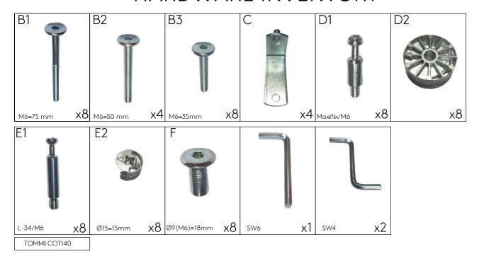
(!) Check hardware against ruler for correct screw. Example Item B2 is 50mm long
