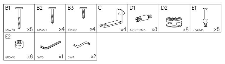
(!) Check hardware against ruler for correct screw. Example Item B1 is 70mm long.
